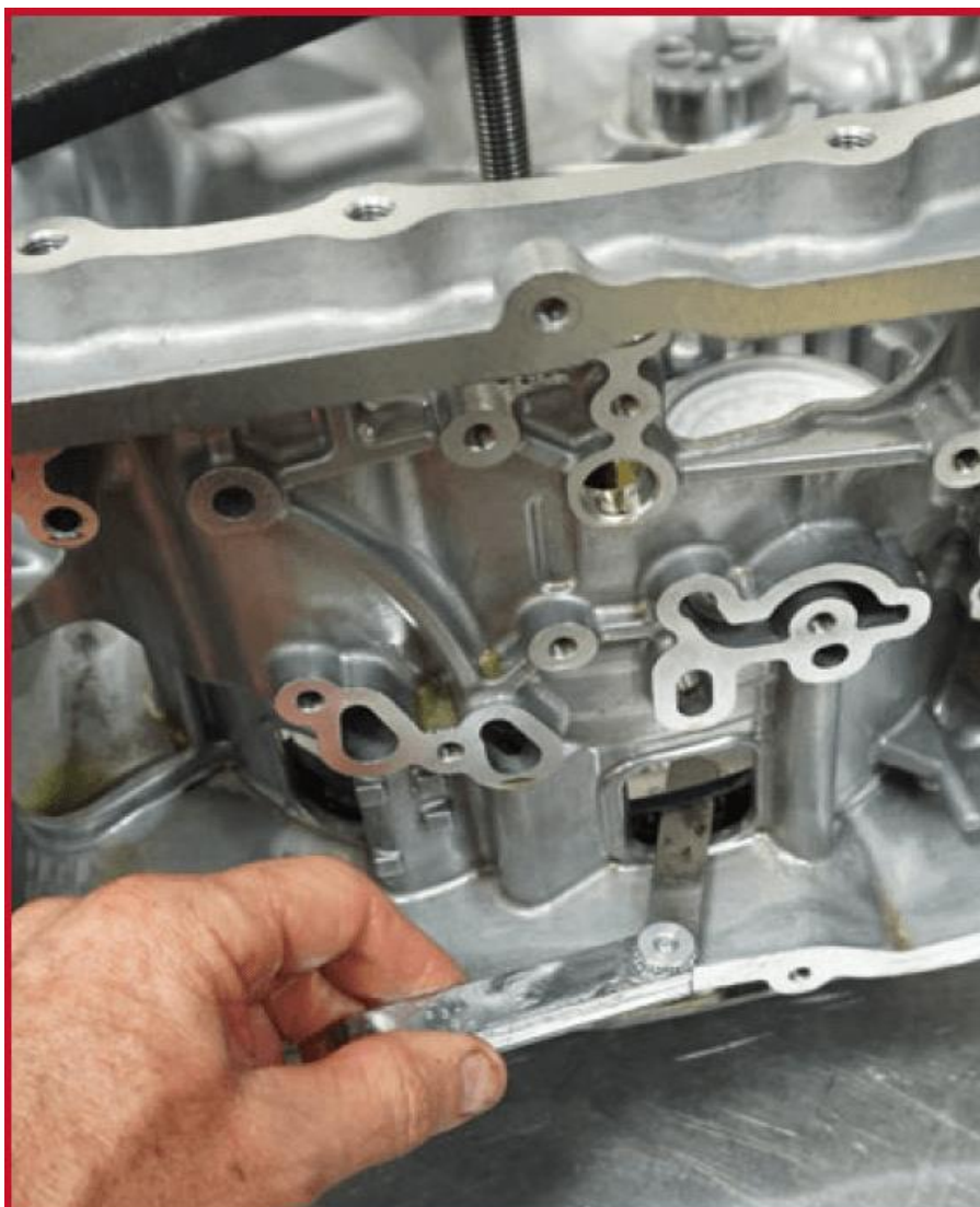
Figure 16: Measure C-Clutch clearance.
