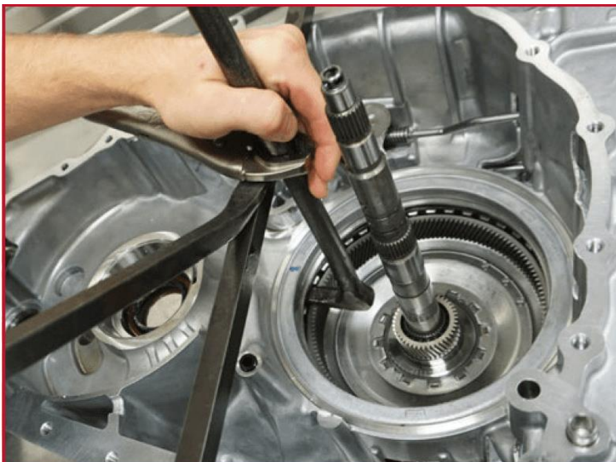
Figure 10: Removing the D-Clutch housing.
