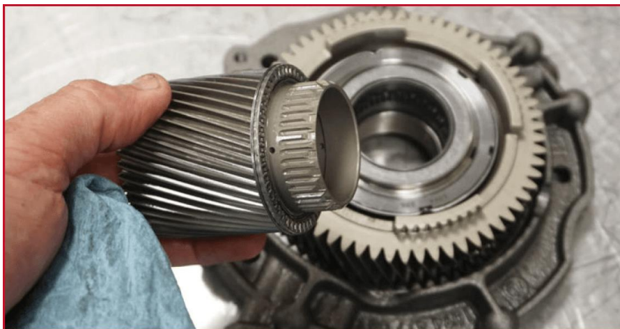
Figure 5: F-Dog locks sun gear to housing.
