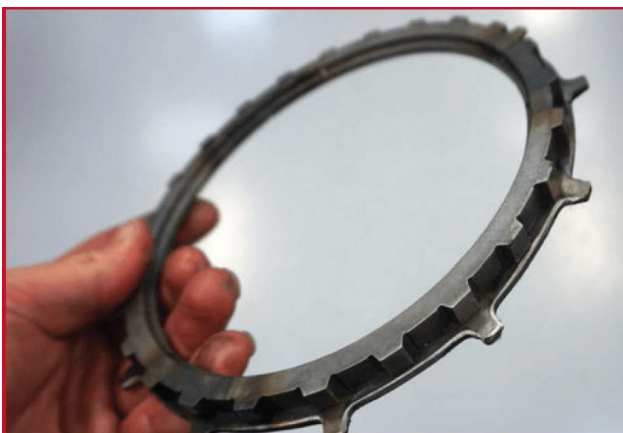
Figure 11: C-clutch spring compressor made from a 6L80 35R steel
