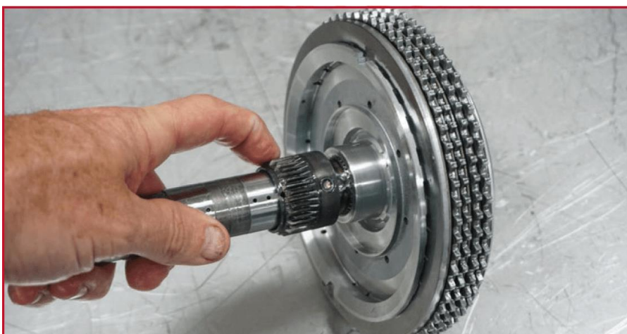
Figure 4: A-Dog Clutch on Input Shaft.
