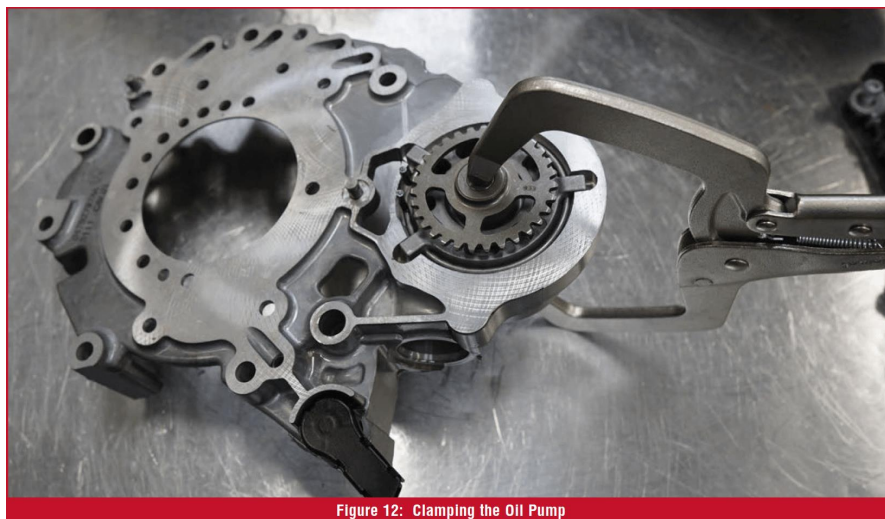
Figure 12: Clamping the Oil Pump
