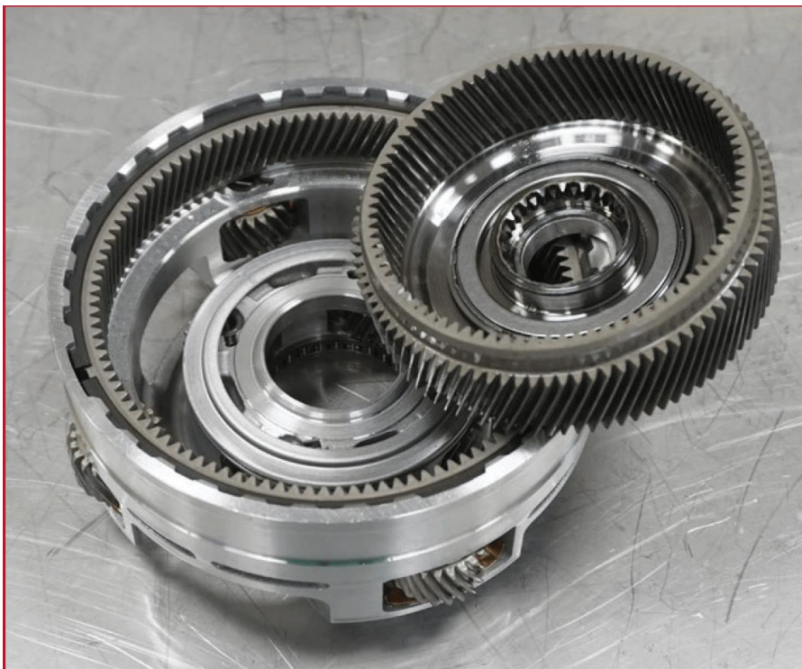
Figure 3: Middle internal and dual rear carrier. Note that the large sun gear is also a small internal gear for the small rear planetary.
