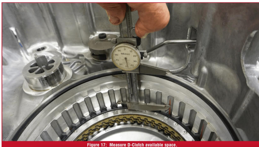
Figure 17: Measure D-Clutch available space.
